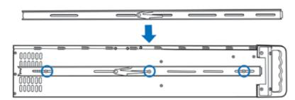
Now put the center slide right next to the rackmount chassis. You should be able to find screw holdes on both sides of chassis. Holes are used for mounting the center slide. Later, the center slide will be use for attaching the sliding rail.
