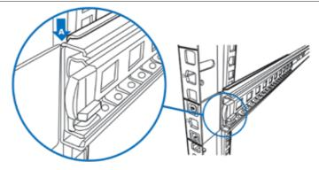
Aline front outter rail to the indent of L bracket between Point A & B.
