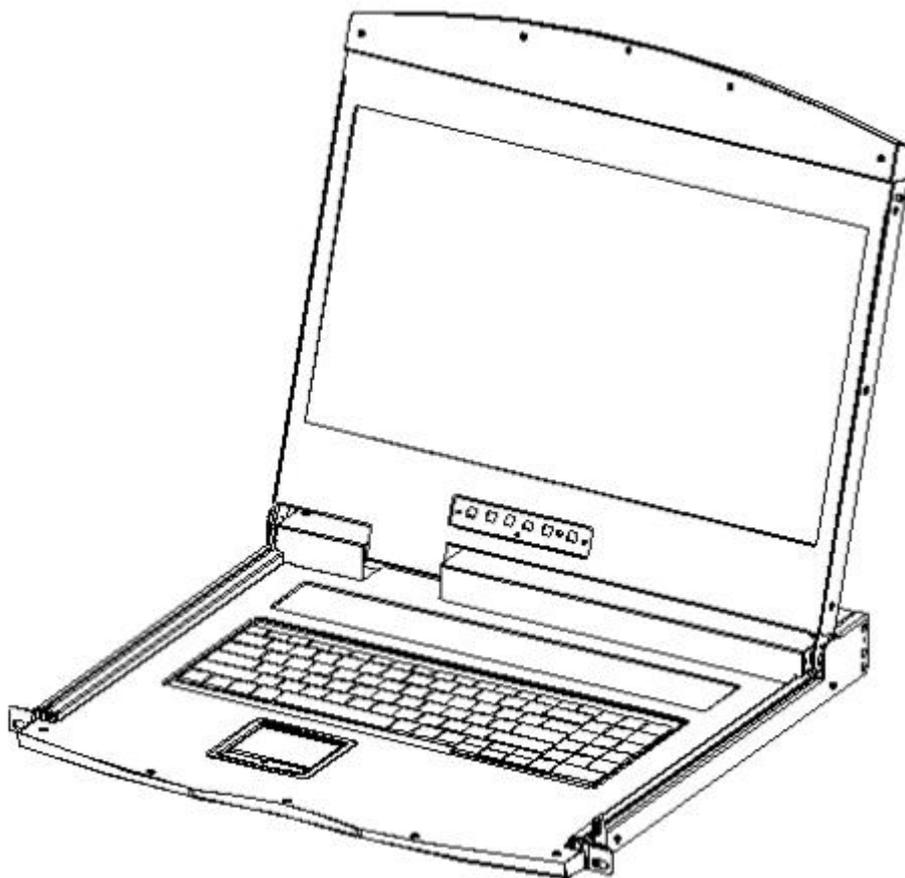
Single-port LCD KVM switch choose KVM cables to connect instead of multi-port use KVM module, divided into two kinds: VGA and DVI according to the port type.
