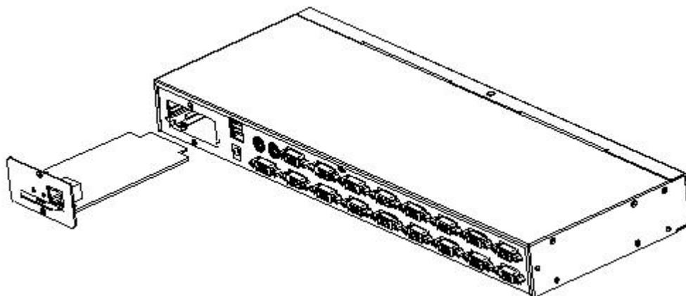
3.After pushing the IP module to the bottom, fix the IP module with the two screws that have been removed before.
