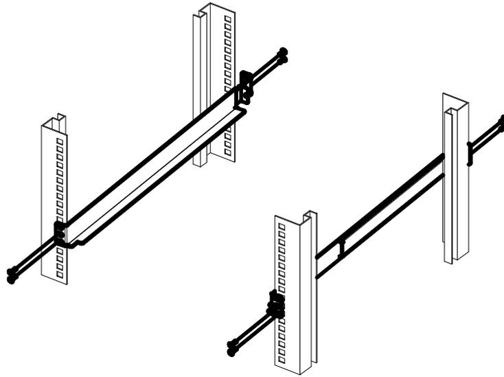
2. Slide the LCD KVM unit onto the support flange, secure the front of the switch to the front of the rack with the screws provided in the package and lock.
