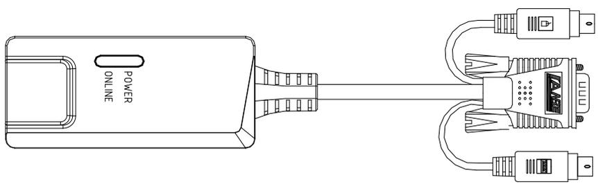
◆ CAT5 connection Dongle VGA + USB (Type A)
