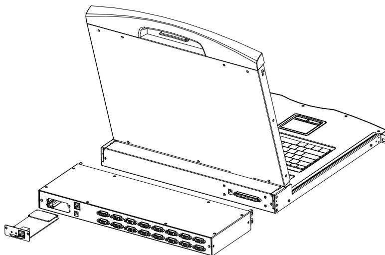
1. find the rear of the device, expansion slot outside the blank position for installation, you need to prepare a screwdriver for removal and installation tools.
