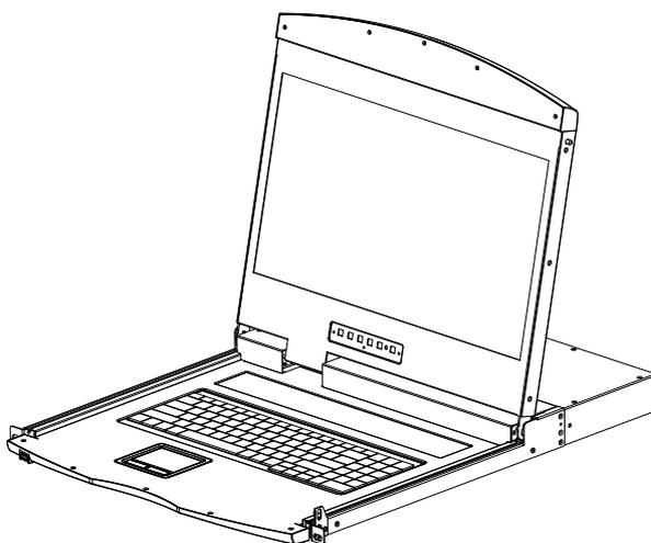
2.The bottom of the keyboard panel has a circular hole, you can use your fingers through the circular hole, the top of the keyboard.
