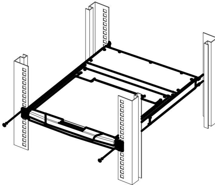
4. Use the screws provided in this package to secure the strip to the rear of the switch. At this point, you have completed the rack mountable LCD KVM switch for subsequent use.
