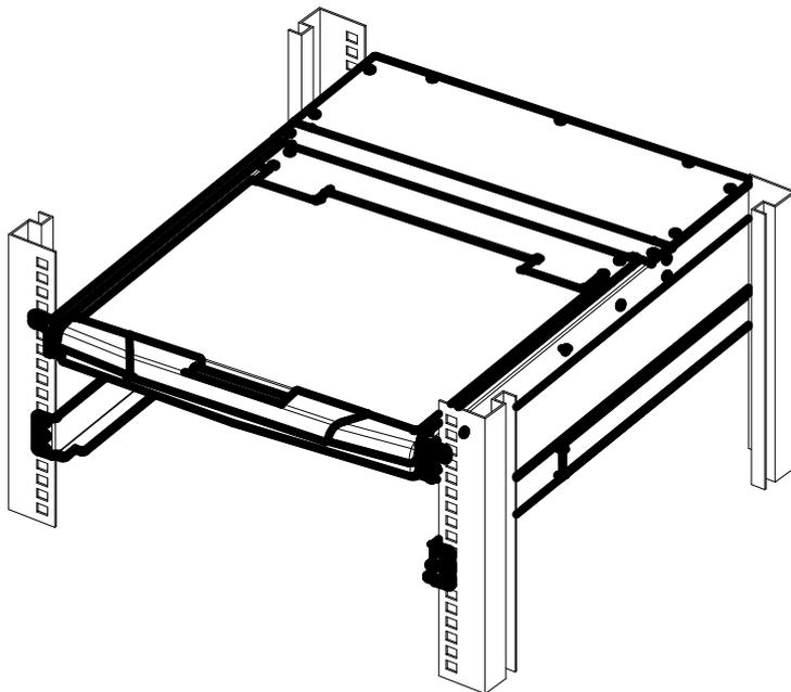
3. Slide the rear connecting slide bracket along the side rails until it reaches the rear of the switch.
