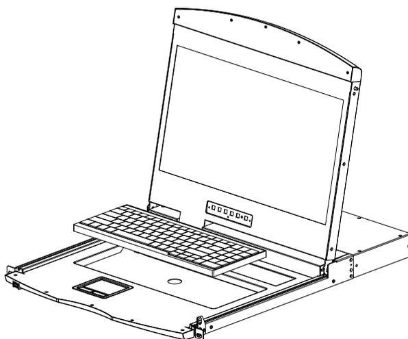
3. Pull the keyboard from the limit slot gently, find the connection side of the USB interface, remove the USB from connection side, the keyboard could be taken out. Thus completing the demolition of the keyboard module.
