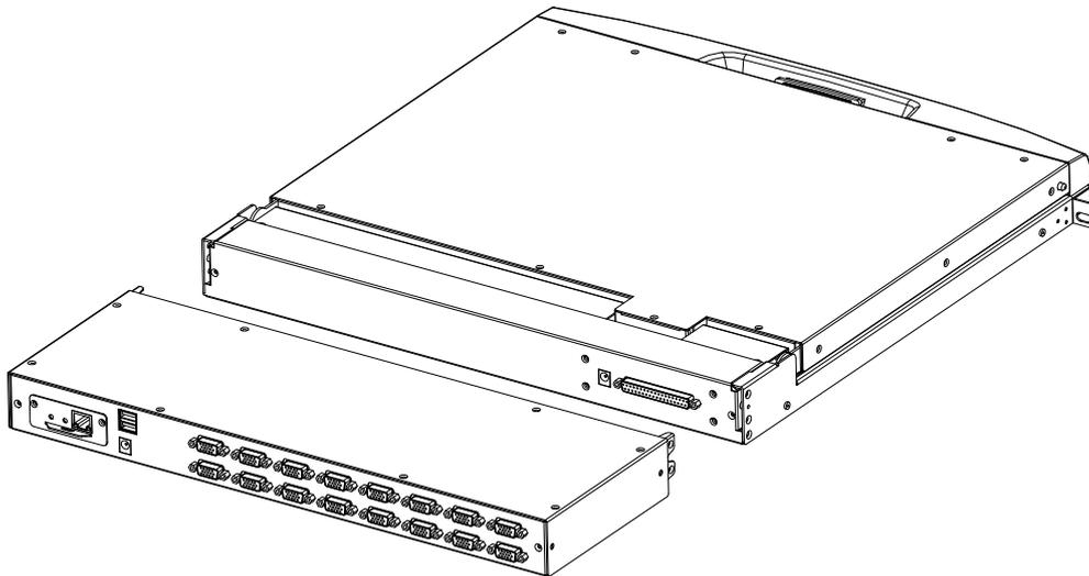
3. Please note the connector between the KVM module & LCD during the Removal and installation, or it may damage the connection interface and equipment function failure.
