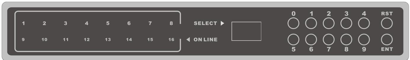
KVM switch button located in the top of the keyboard operating area, divided into three blocks, from left to right in order is the online indicator display area, Port switch to select the display area, Port switch digital button area.
