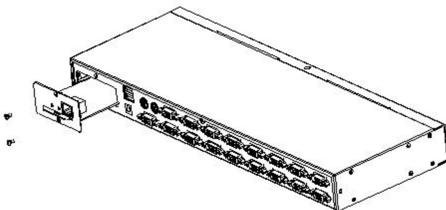
4.After installing the IP module, you need to follow the instructions of the IP module To install the software and configure the IP address of the device before you can connect the network cable to the switching device. After the installation is complete, you can access the network to log in. (For details, refer to the IP module's product manual.)
