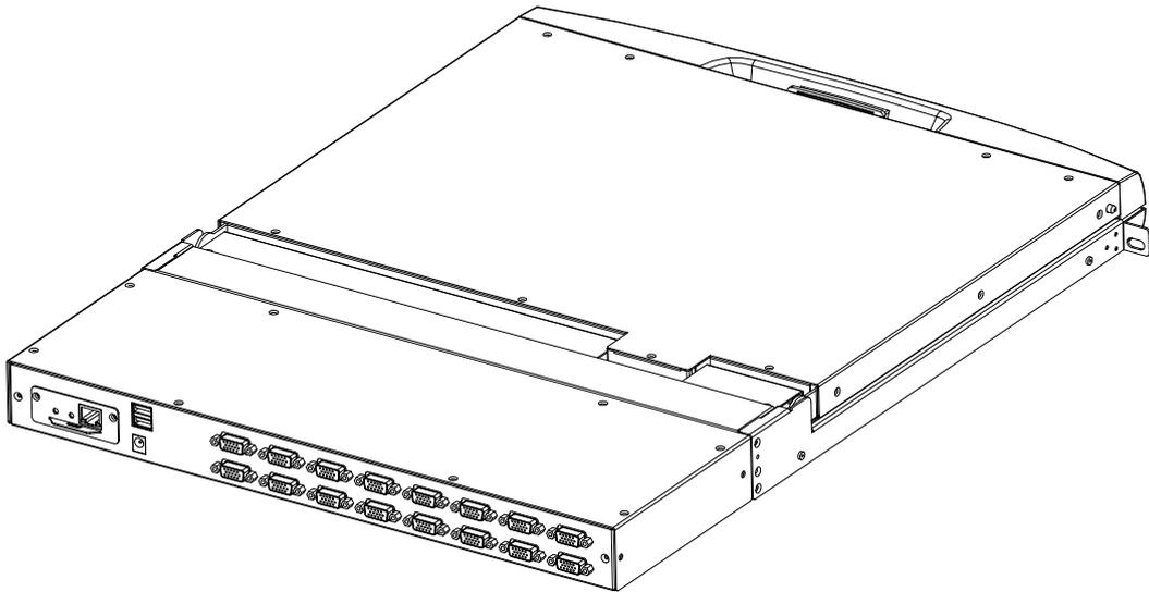
2. Remove the KVM assembly and the captive screws on the side brackets as shown to separate the KVM assembly from the front LCD assembly.
