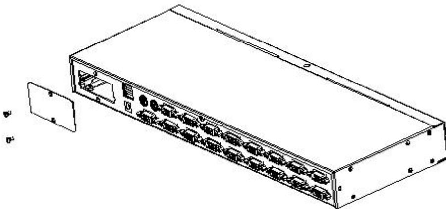
2.Remove the extended IP module and push it gently into the recess in the mounting module cavity as shown.
