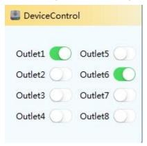
This window allows users to manually turn the power on or off.
