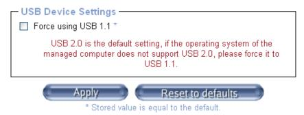
USB 2.0 is the default setting, if the operating system of the managed computer does not support USB 2.0, please force it to USB 1.1.
