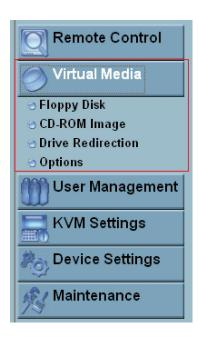
Drive Redirection allows you to share (redirect) your local drive (floppy drives, hard disks, CD ROMs and other removable devices like USB sticks) with the remote system over a TCP network connection. Thus, with Drive Redirection, you can use a virtual disk drive on the remote computer instead of an image file. It is also possible to enable a remote machine to write data to your local disc.
