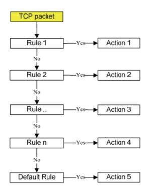
Figure 67: Chain Rules of IP Filtering
