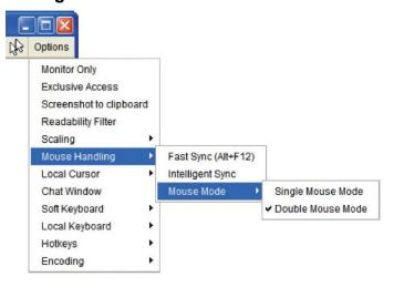
The submenu for mouse handling offers two options for synchronizing the local and the remote mouse cursors.
