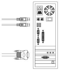
Figure 8: PS/2 (Keyboard & Mouse) and VGA connected
