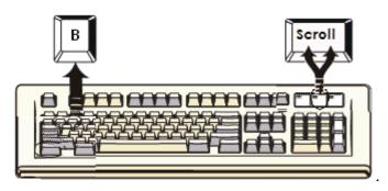
Figure 13: Buzzer setup hot key
