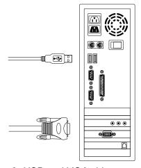
Figure 9: USB and VGA video connected
