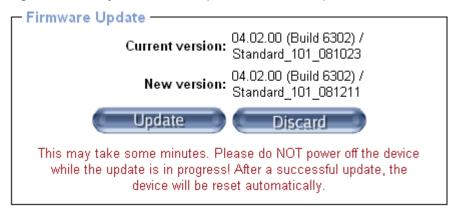
The panel shows you the version number of the currently running firmware and the version number of the uploaded firmware. Pressing **Update** will store the new version and substitute the old one completely.
