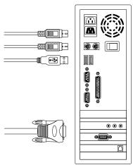
Figure 7: USB & PS/2 (Keyboard & Mouse) and VGA connected
