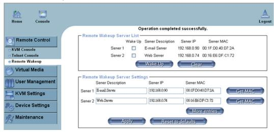
The IP-KVM provides the remote power wakeup function, which can remotely wake up the sleeping computer. With this feature, the computers that are not in use for now can be shut down and remotely wake up the computer when want to use it, and thus save the power energy.
