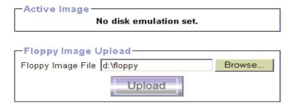
Click on the button **Upload** to initiate the transfer of the chosen image file into the IP-KVM module's on-board memory
