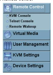
The Remote Console is the redirected screen, keyboard and mouse of the remote host system that IP-KVM controls. The Remote Console window is a Java Applet that tries to establish its own TCP connection to the IP-KVM.
