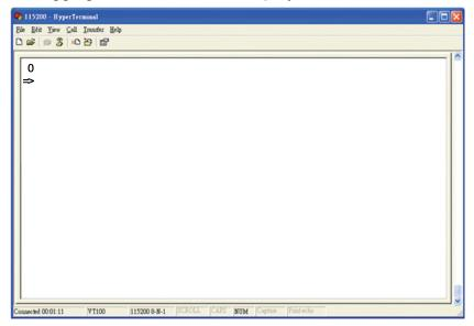
3. Key in "defaults" command and then Enter. The unit will automatically set to factory default settings and reboot the system.
