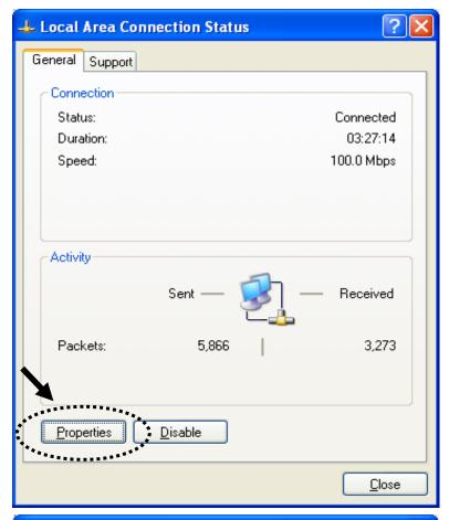
1. Set your computer to obtain an IP address from wireless router: click 'Start' button (it should be located at lower-left corner of your computer), then click control panel. Double-click **Network Connections**, then double-click **Local Area Connection**. Click 'Properties'.
