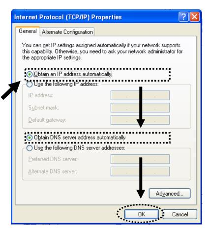
3. Select 'Obtain an IP address automatically' and 'Obtain DNS server address automatically', then click 'OK'.
