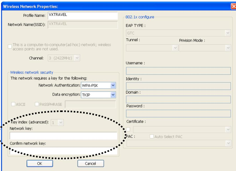
4. If a password (a.k.a. 'Network Key') is required to access the wireless access point, please input it in 'Network key' (and input it again in 'Confirm network key' for confirmation). Click 'OK' when password is properly inputted.
