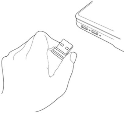
1. Insert the USB wireless network card into an empty USB 2.0 port of your computer when computer is switched on.
