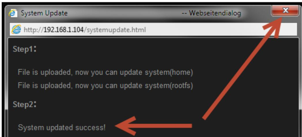
... close this window. In the system menu of the camera interface click on "Reboot" and confirm whether the camera should be rebooted with "OK".
