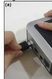
10a. If would like to use eSATA cable, plug eSATA cable into the HD enclosure
