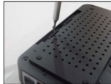
6. Securely tighten screws from the bottom of HD enclosure to fix hard disk (4pcs short screws)
