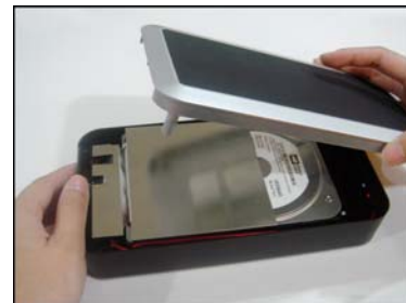
8. Replace cover onto HD enclosure
