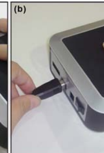
10a. If would like to use eSATA cable, plug eSATA cable into the HD enclosure
