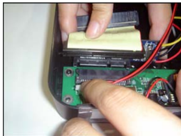
3. If would like to use PATA hard disk, please connect little PCBA with big PCBA
