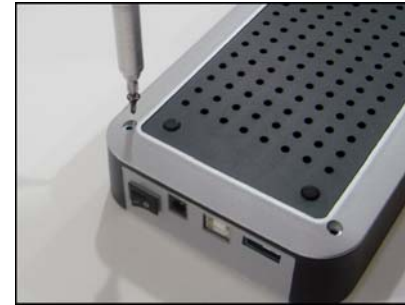
9. Use screws (2pcs longer, 2pcs shorter) from the bottom of HD enclosure to tighten it
