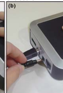
11a. After plugging eSATA cable into the HD enclosure, plug adapter into HD enclosure
