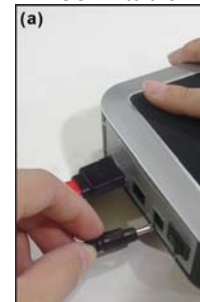
11a. After plugging eSATA cable into the HD enclosure, plug adapter into HD enclosure
