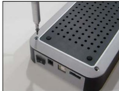
6. Use screws (2pcs longer, 2pcs shorter) from the bottom of HD enclosure to tighten it
