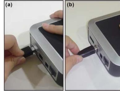
7a. If would like to use eSATA cable, plug eSATA cable into the HD enclosure
