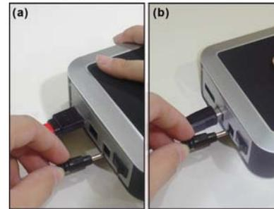
8a. After plugging eSATA cable into the HD enclosure, plug adapter into HD enclosure
