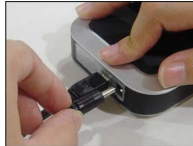
8. If additional power is needed, plug DC power into HD enclosure
