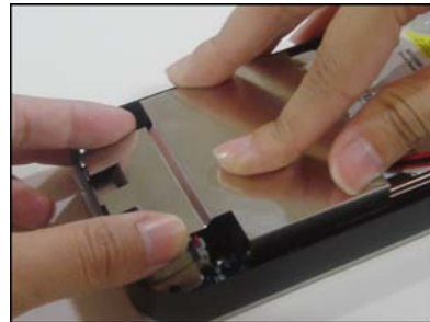
5. Assemble PCB shielding above PCBA
