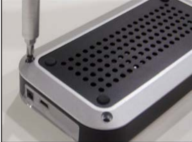
6. Use screws (2pcs longer, 2pcs shorter) from the bottom of HD enclosure to tighten it
