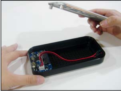
1. Carefully remove cover from HD enclosure
