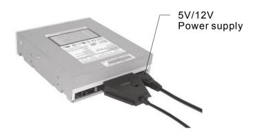
For a 5.25 CD/DVD device, plug directly the 40pin connector into the appropriate ports on the rear of the CD/DVD device, and plug the USB signal/data plug (Black) into USB port of PC, then plug the 4-pin plug of the power supply to the 4-pin power jack (for IDE CD/DVD direct plug in CD/DVD power connector), and the other end plug to power source.
