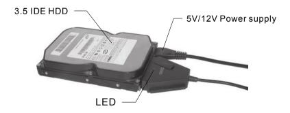
For a 3.5 SATA HDD or a 3.5 IDE HDD, plug directly the SATA connector or the 40pin connector into the appropriate ports on the rear of the HDD, and plug the USB signal/data plug(Black) into USB port of PC, then plug the 4-pin plug of the power supply (not included) to the 4-pin power jack (for IDE HDD direct plug in HDD power connector), and the other end plug to power source.
