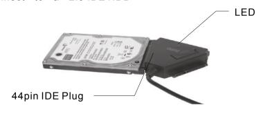
For a 2.5 SATA HDD or IDE HDD, plug directly the SATA connector or the 44pin connector into the appropriate ports on the rear of the HDD, and plug the USB signal/data plug (Black) into USB port of PC.
