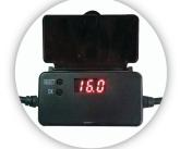
4.when the flashing data show the output voltage correspond to the value of your label .Press ok
